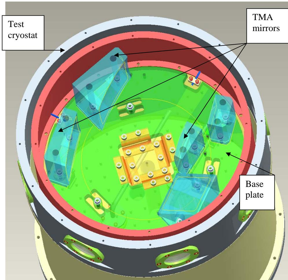
Figure 16: METIS prototype TMA mounted in the test cryostat
