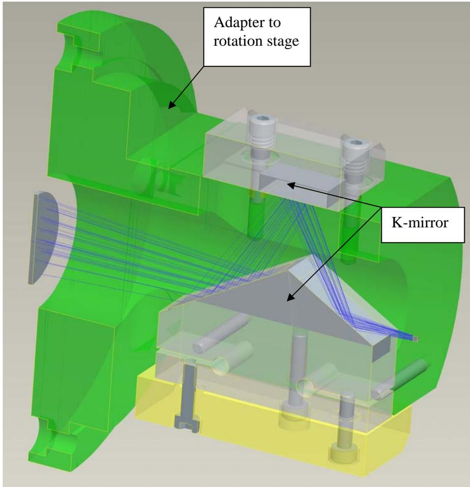
Figure 17: Image derotator (K-mirror) for GRAVITY wavefront sensor
