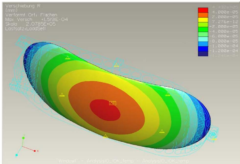
Figure 3: FEM simulation of the main mirror with 50  $\mu\text{m}$  NiP-layer, radius deviation: 160 nm @  $\Delta T=10$  K
