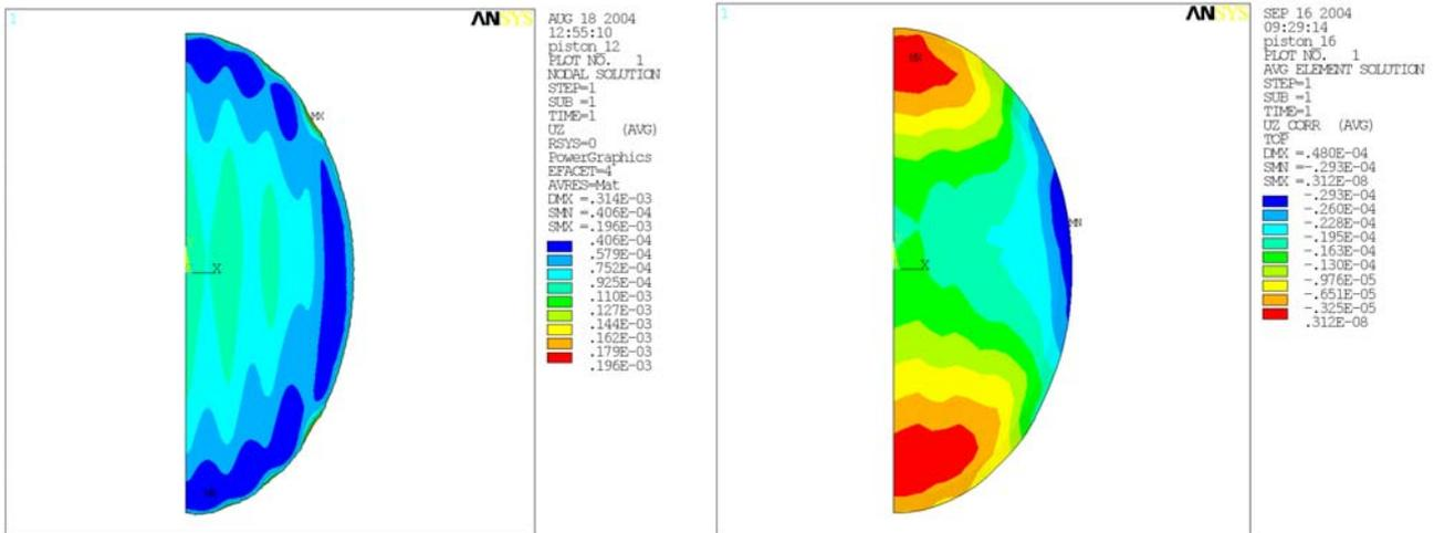
Figure 2: Mirror Al 6061 (left = 66 nm p-v) and AlSi (right = 39 nm p-v) with a 50 µm NiP layer at ΔT = 25 K (simulation)
