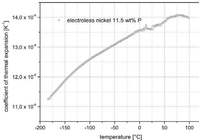
Figure 10: CTE Measurement on an electroless nickel tube
