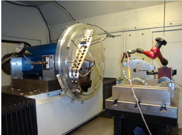
Figure 4: Diamond turning of the main mirror
