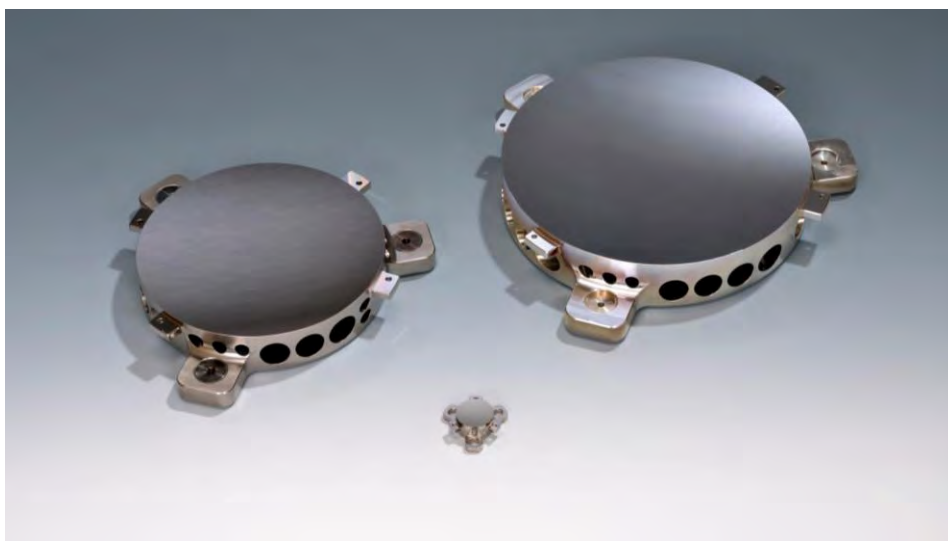
Fig. 5. Metal optics for the PCW Mission: primary mirror (left), secondary mirror (center), tertiary mirror (right), with AlSi40 as substrate material and electroless nickel (NiP) as polishing layer.
