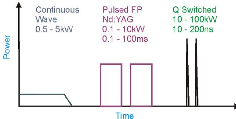
Figure 1 Schematic representation of the output characteristics of various welding laser sources, with peak power and pulse durations ranges where relevant. The FP Nd:YAG laser combines high peak power with sufficiently long pulse widths for usable energy for exceptional spot welding and low heat input seam welding.
