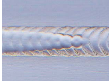
Figure 3 Fadeout capability on seam welds, to prevent last pulse cracking and ensure completion of smooth seam.
